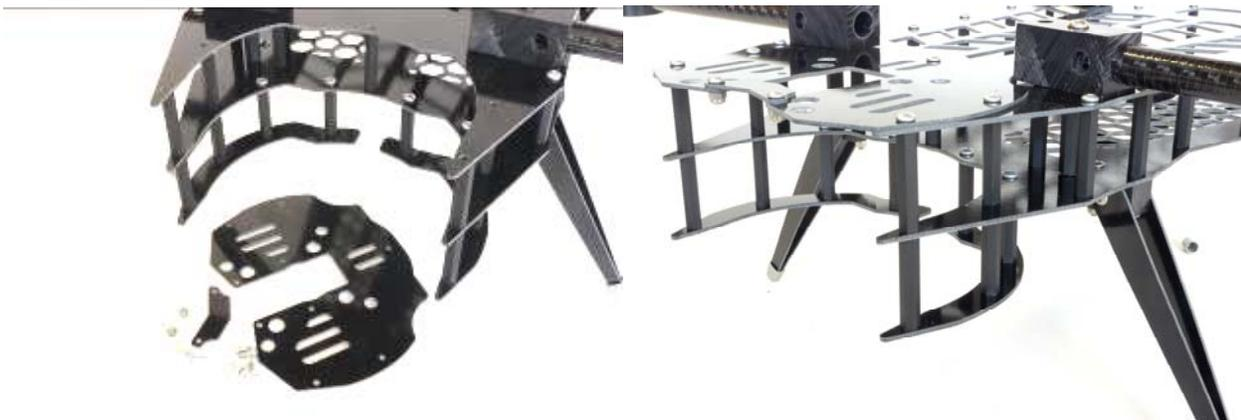
IT places your expensive camera/gimbal assembly in a protective cage. This gimbal and plate assembly can be changed out in minutes with another camera and gimbal. Keep multiple gimbal/camera assemblies on hand and exchange with just 5 screws. Buy inexpensive blank plates and custom drill them to suit.
