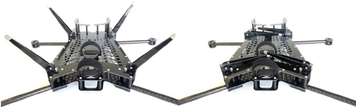
IT has folding landing gear that "give" to absorb shock during a hard landing - easy and inexpensive to replace in the field.
