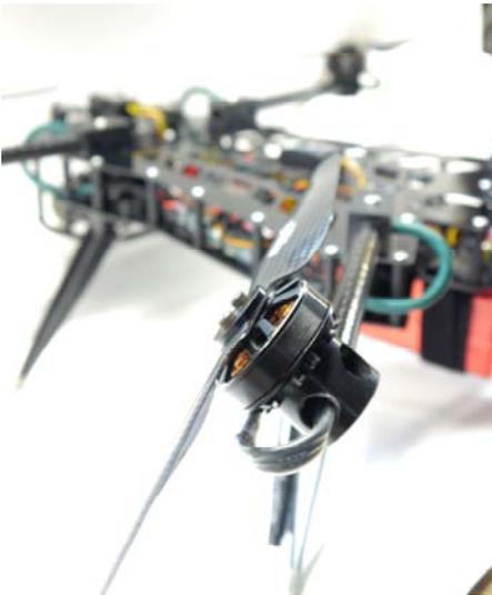
IT has press fit, indestructible Delrin motor mounts that rotate in a crash to save your motors.
