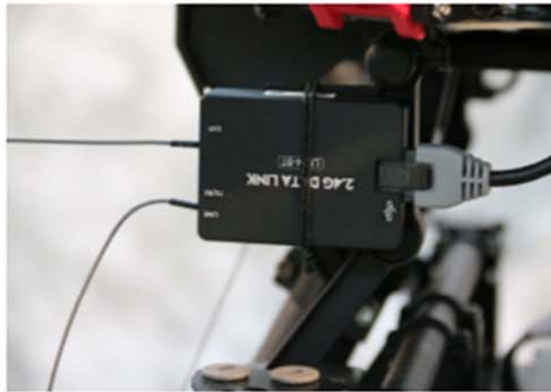
Ground Station 2.4GHz Remote Unit
