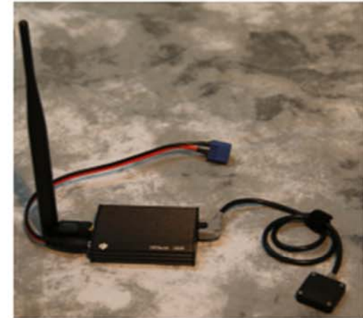
Ground Station 2.4GHz Blue Tooth Unit, connects with iPad
