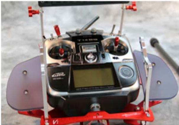
Futaba 14SG with SE Craft Aluminum tray with monitor mount and side pads
